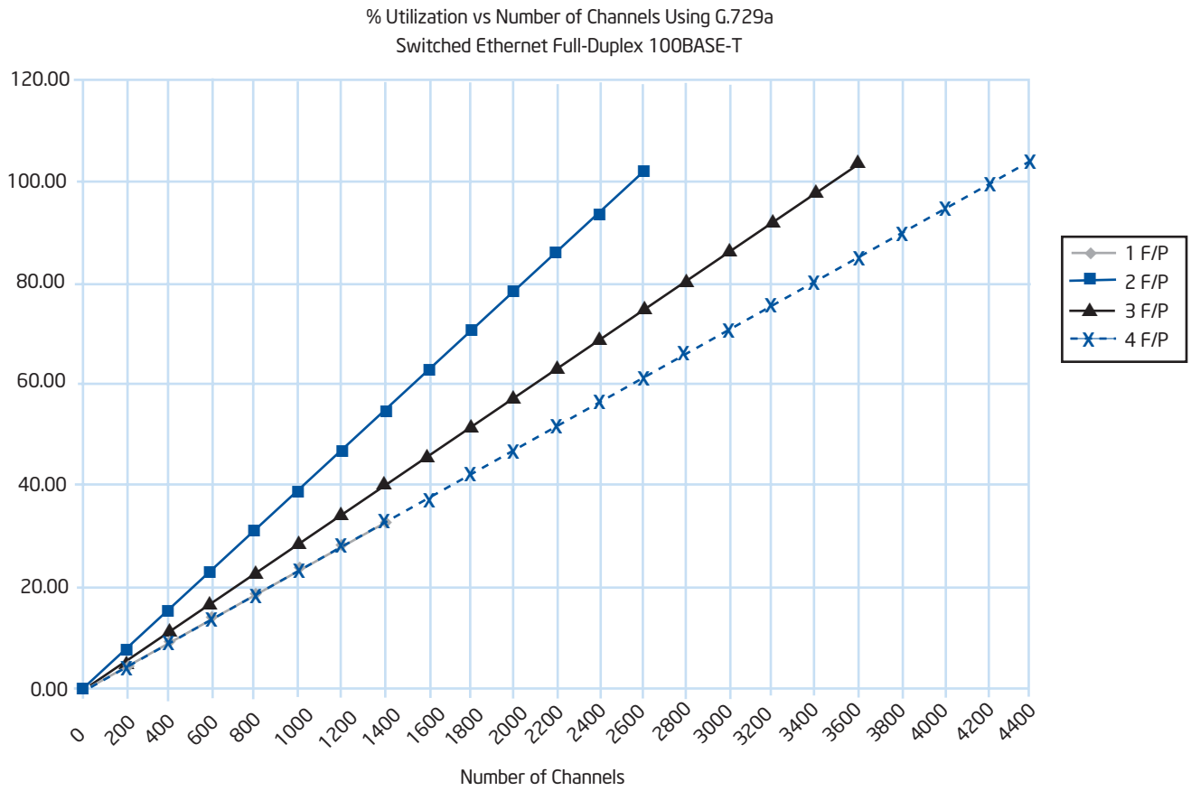
Figure 19. Utilization vs. Number of Channels for G.729
